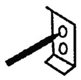
1. Hold accessory to desired location on wall. Mark wall for mounting brackets.
