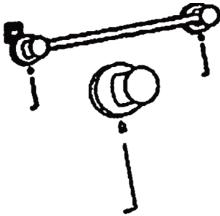
5. Secure accessory to bracket using set screws and allen wrench provided.
