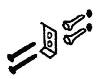
3. Screw mounting brackets securely to wall.
